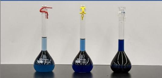
Photograph showing three volumetric flasks containing the molybdenum blue complex, demonstrating the color change from light blue to dark blue as the concentration of  $\text{PO}_4^{3-}$  ions increases.
